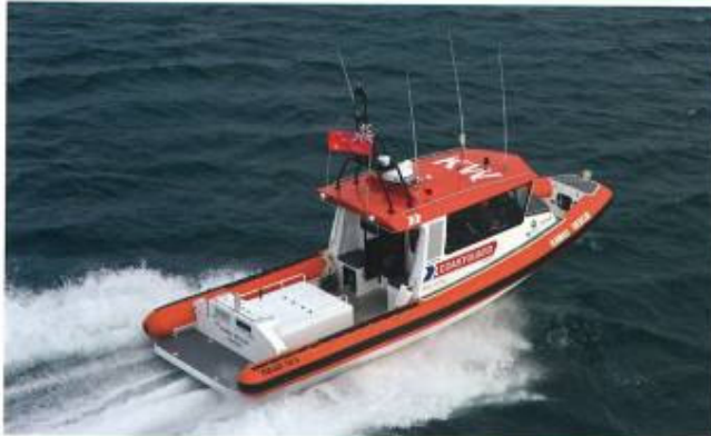
'Kawau Rescue' is a 10.2-metre Nalad RIB built by Blue Water Boats and propelled by twin HamiltonJet HJ274 waterjets.
